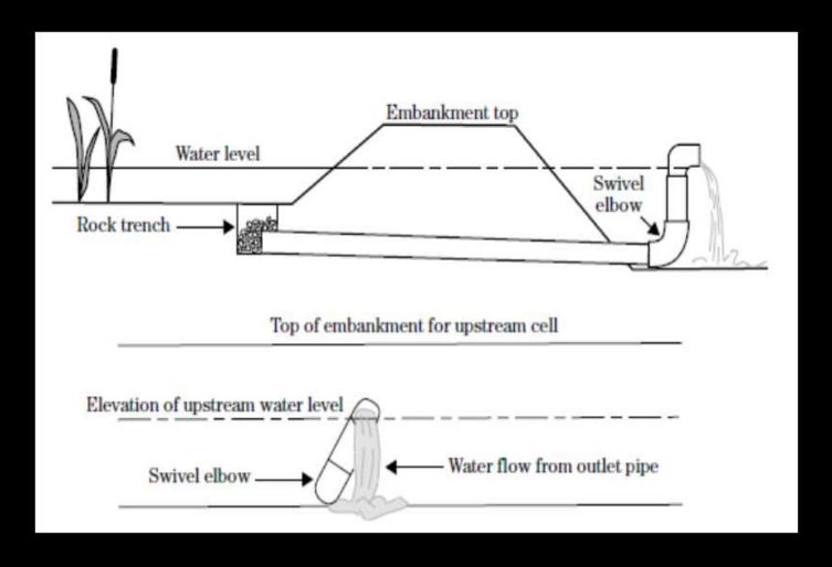
In other words, water level in the upstream cell will be at the same elevation as the invert of the downstream outlet pipe.
